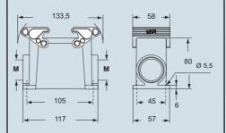
The surface mounting, high construction housings are supplied with an open threaded entry and diametrically opposite a closed threaded entry which can be opened by the user if required (with suitable tool).
