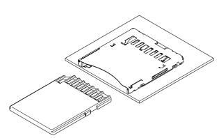
This connector is designed for SD Card & MMC (Multi media card), complying with the SD Card Association standard, and is with the switch for Write-protection & Carddetection. And due to Push-push mechanism design, its card can be easily ejected by push-push operation.
