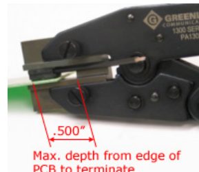
Figure 2: Wire Placement in Tool
