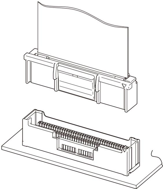
**This connector realizes high cost performance, to be designed with the new connector concept that the conductors of flat cable that was fixed up in the plug housing are directly touched to the base contacts.**
